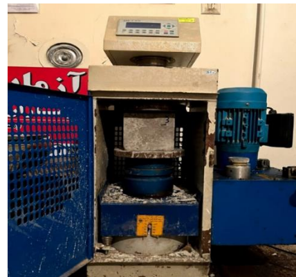
Figure 5: Jack for compressive strength testing
