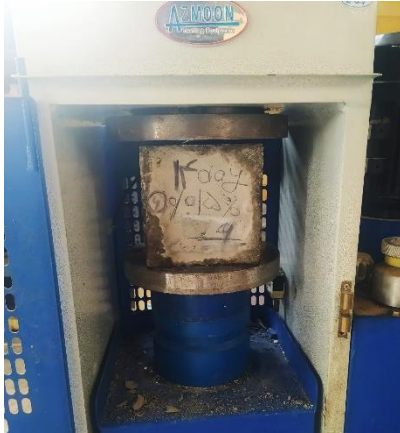
Figure 6. Compressive strength test on cubic sample
