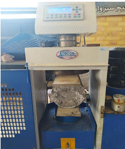
Figure 8. Testing the tensile strength of the cylindrical sample
