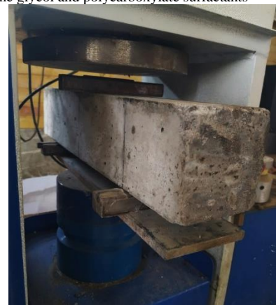
Figure 10. Flexural strength test of prismatic beam
