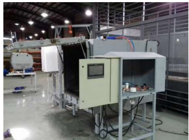
Figure 2. In-vessel composting reactor pilot plant.
