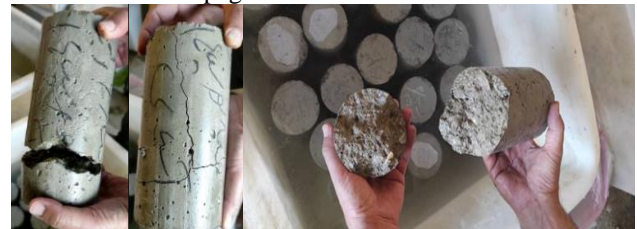
Figure 5. Loss of strength and disintegration of concrete specimens cured using a pond with stagnant, non-replaceable water after 120 days.
