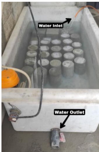
Figure 3. Sample storage pond with temperature control and replaceable water
