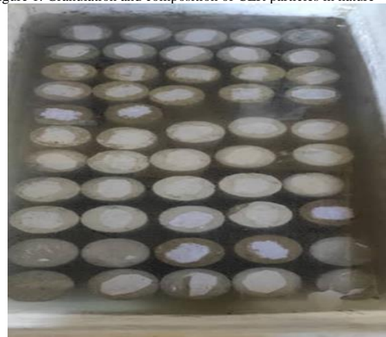
Figure 2. Sample storage pond with stagnant and non-replaceable water
