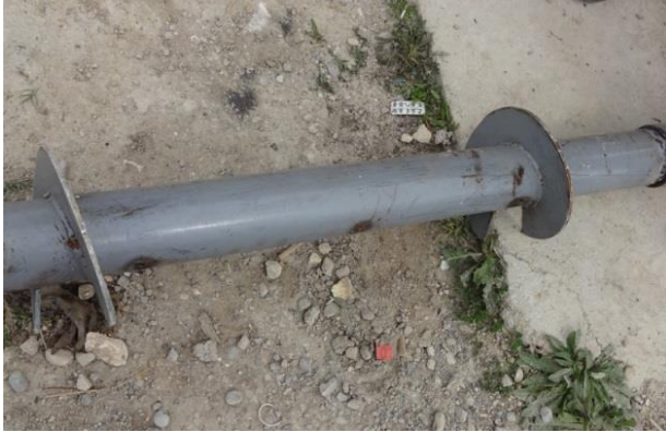
Figure 4. The double helix pile used in this study
