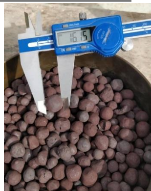
Fig. 2. Iron mill scale and Iron pellets shapes and sizes.
